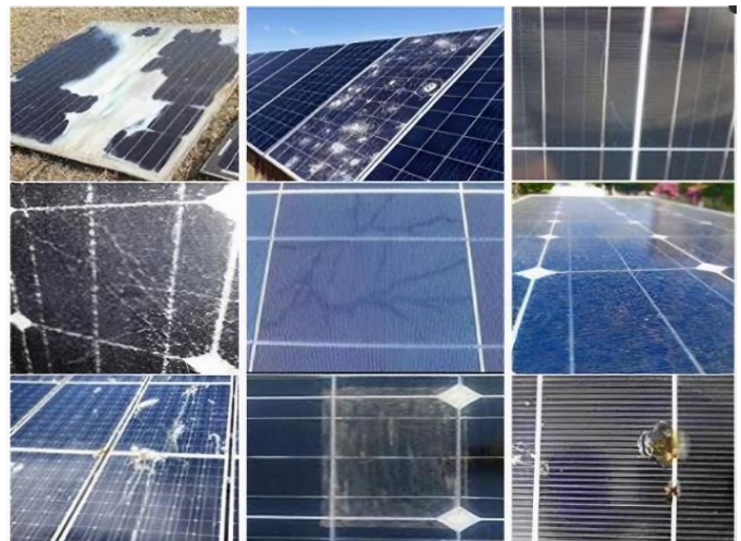
Figure 2. Representative Examples of Common Surface Defects Observed in Solar Panels, Including Dust Accumulation, Bird Droppings, Snow Coverage, Physical Damage, And Electrical Damage.
